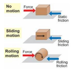
a) Static friction: is the friction that prevents an object from moving when it is at rest. It acts between two surfaces that are not moving relative to each other. This force must be overcome to start the motion of the object.
